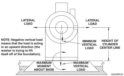
The moment about the base reciprocates and would cause a "rocking" motion if any of the following conditions exist:
